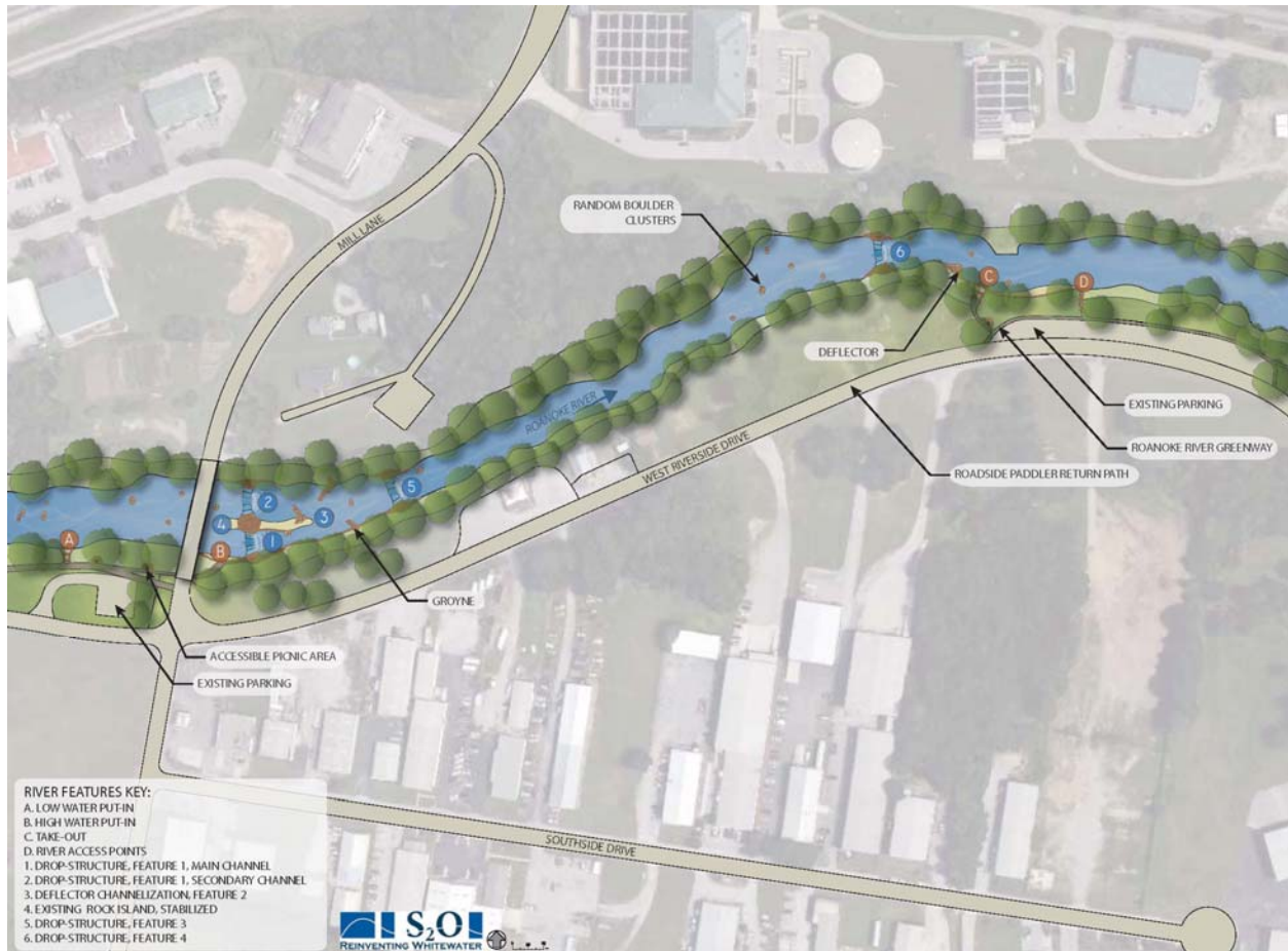
Figure 10: The conceptual design for the Mill Lane Site
