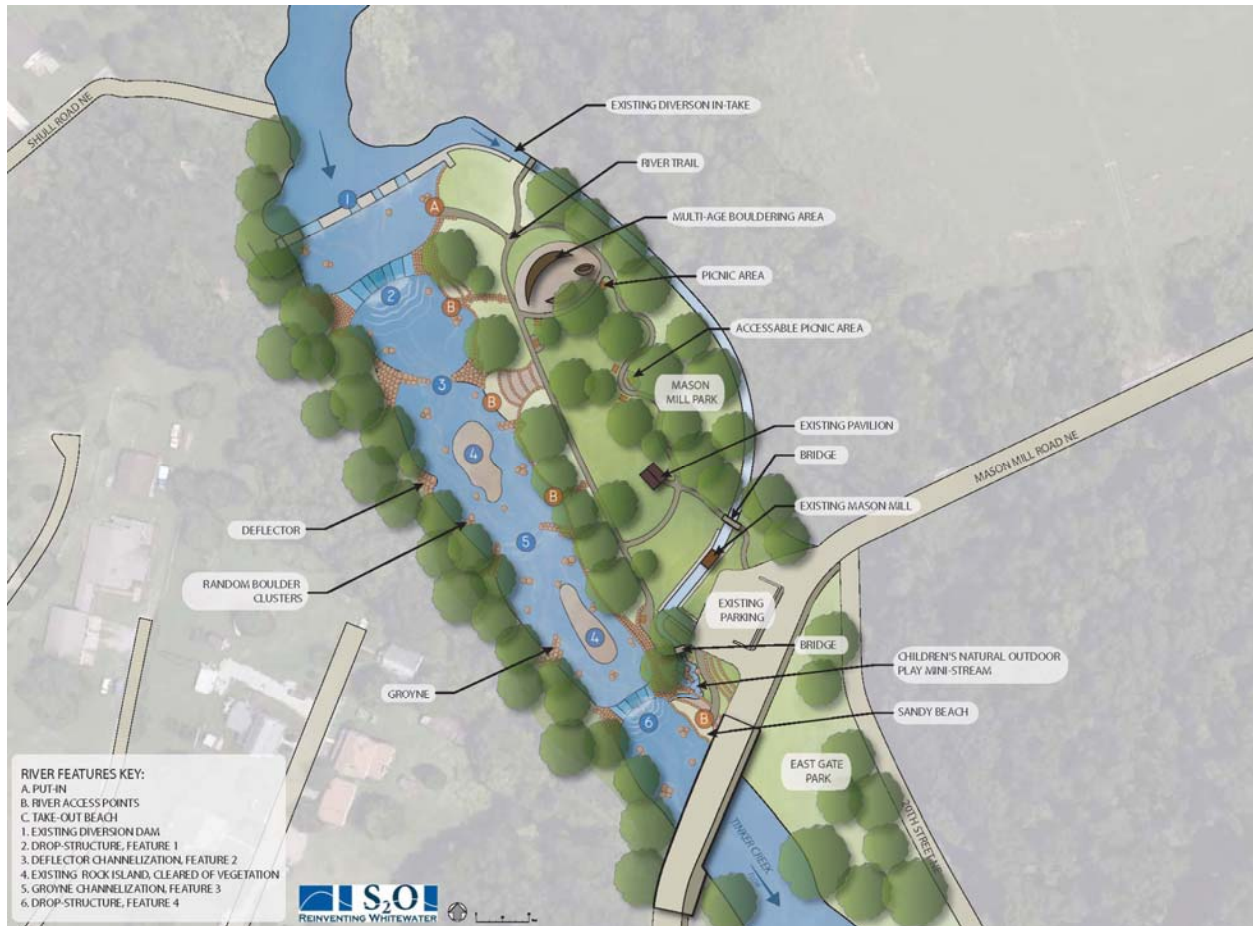
Figure 33: The conceptual design for the Tinker Creek Site.
