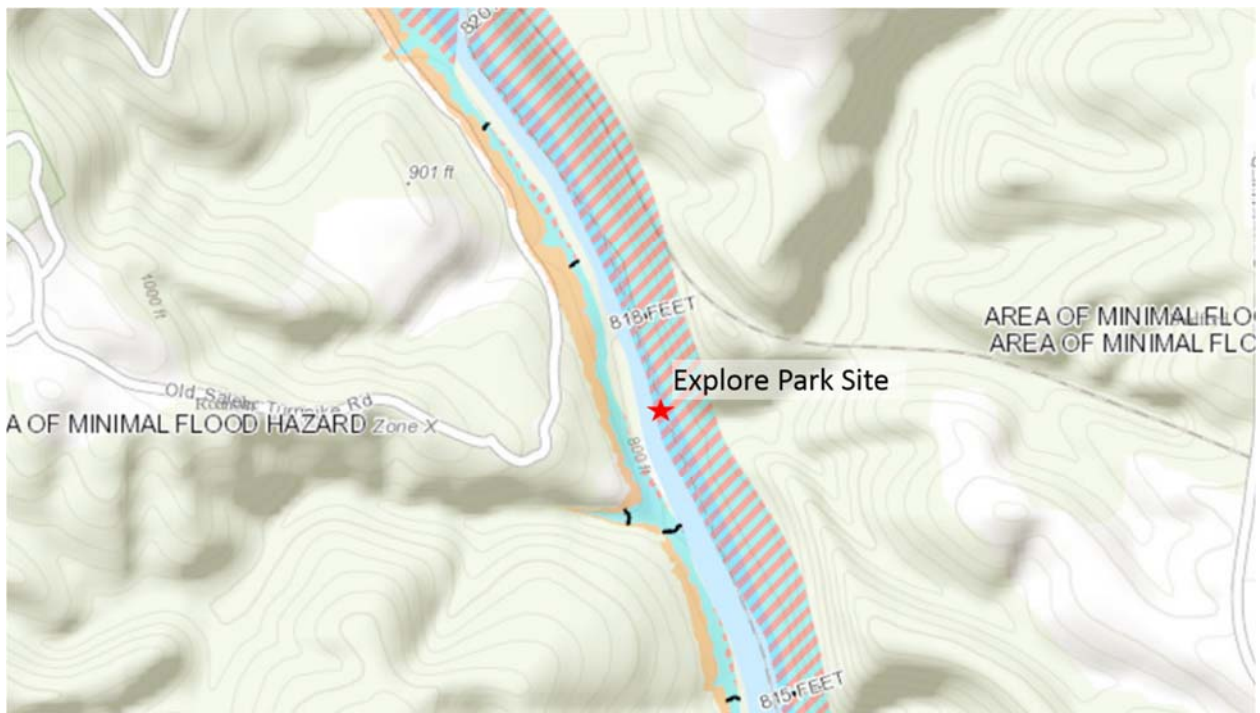
Figure 25: FEMA Flood Hazard Mapping for the Explore Park project site (FEMA's National Flood Hazard Layer (Official), 2015).
