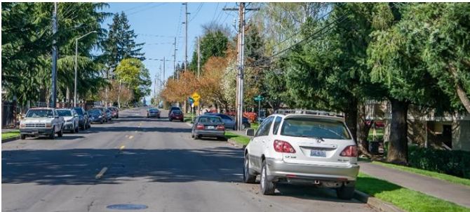
Figure 10: Northeast 72nd Avenue near Northeast 55th Street has two travel lanes with shoulders that are used as parking.
