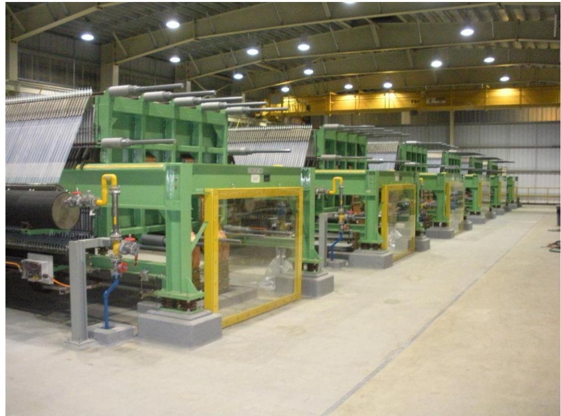
A look at the cell room in North Vancouver, which contains the specialized units where chlorine is created
