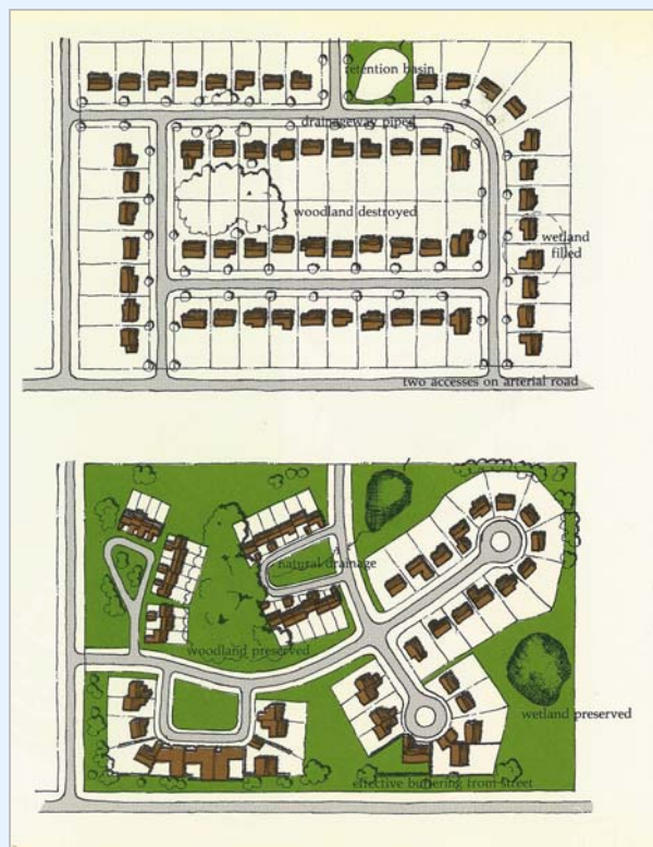
Figure 3.1 Development clustering as shown in the lower example is an alternative approach for conventional subdivision development (displayed in the upper example), which allows an equivalent density while conserving natural resources, preserving open space, and protecting recharge zones.
