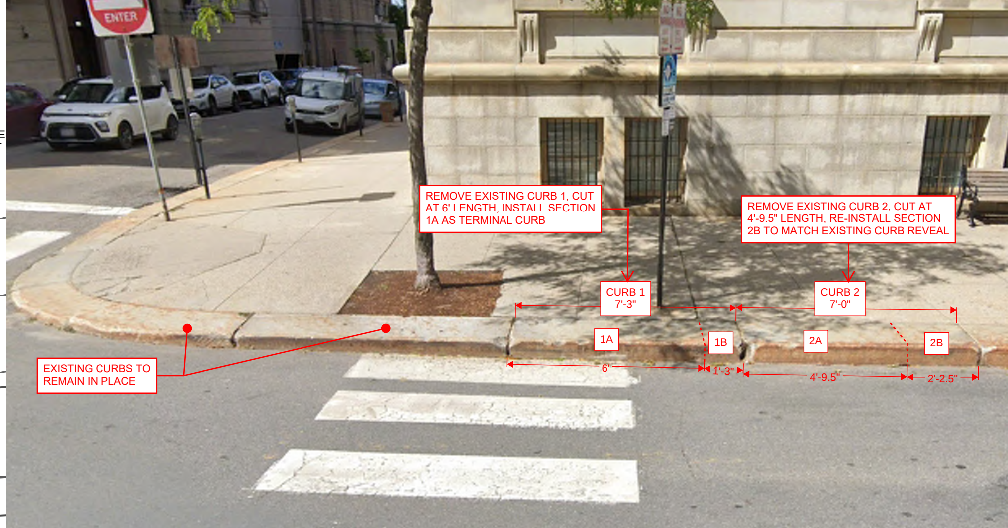
FIGURE 3: CURB MODIFICATION PLAN
