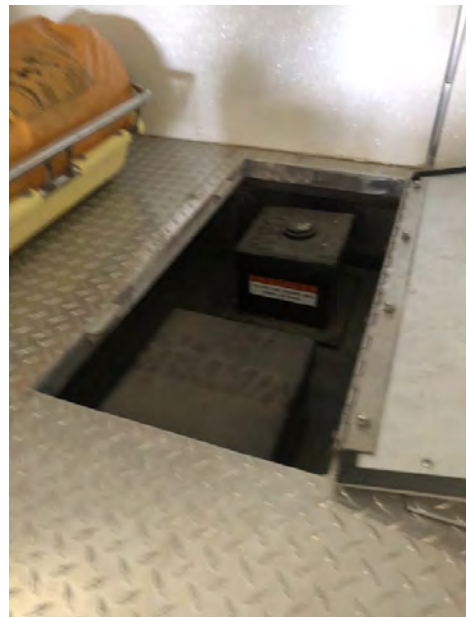
AFFF concentrate tank on rescue truck
