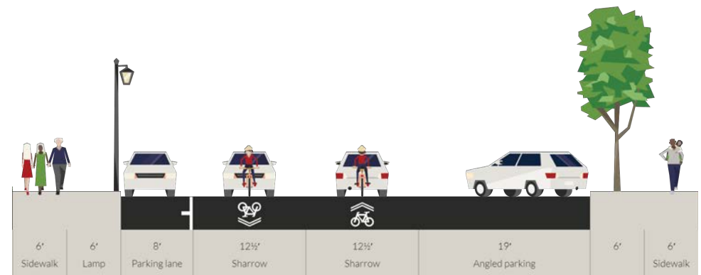
Figure 69: Section FF on Main Street for alternative M4 (outside of Rite Aid)
