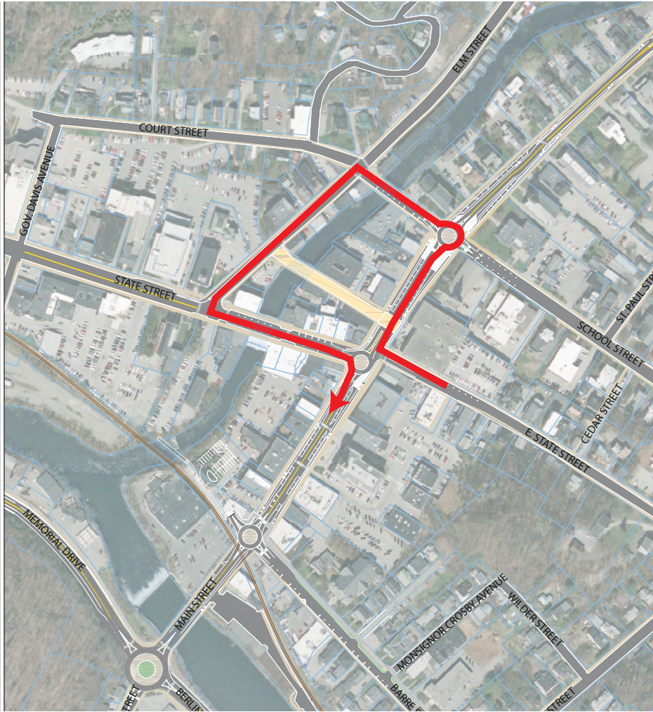
Figure 60: Route for all vehicles wanting to turn left from East State Street to the southern portion of Main Street. According to traffic data from VTrans, approximately 43% of the westbound traffic on East State Street turn left onto Main Street (approximately 775 vehicles per day; the AADT of School Street in 2013 was 1800).
