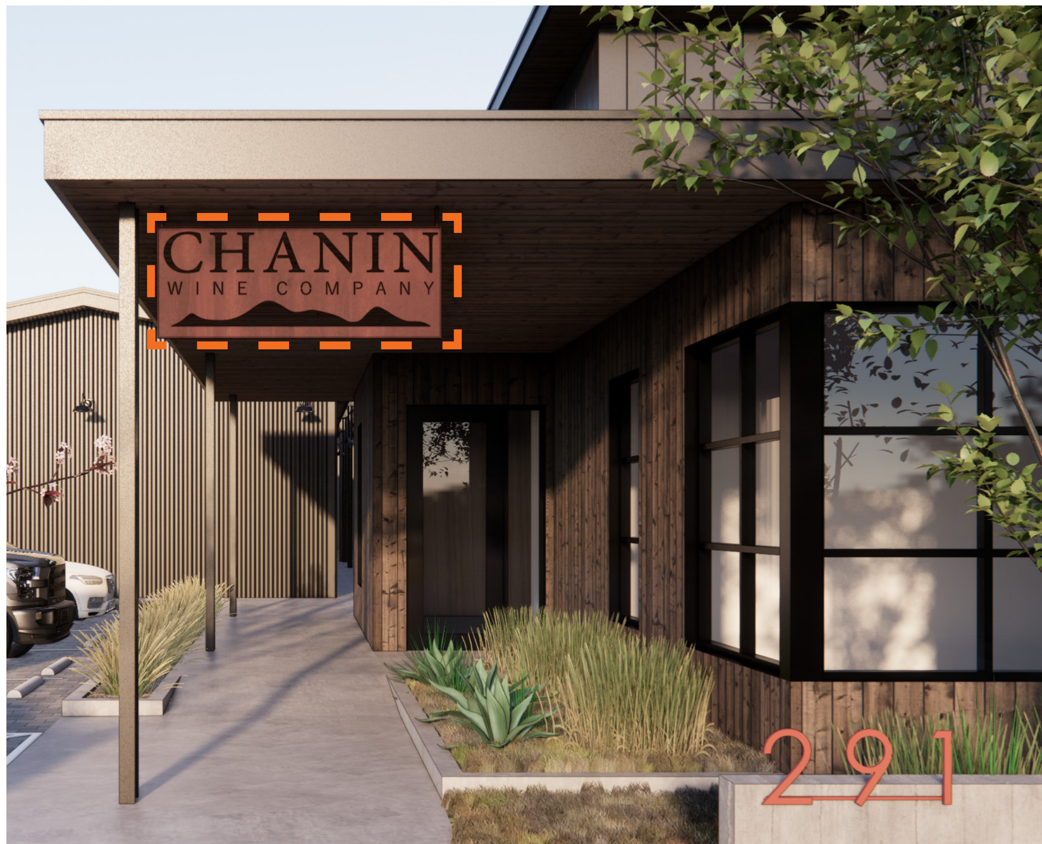
SUSPENDED SIGN #1 5'-0" wide x 2'-0" tall cut steel logo lettering with recessed directional accent lighting in the eave above 10 sf sign area 9' clearance exceeds 8' minimum required above pedestrian areas
