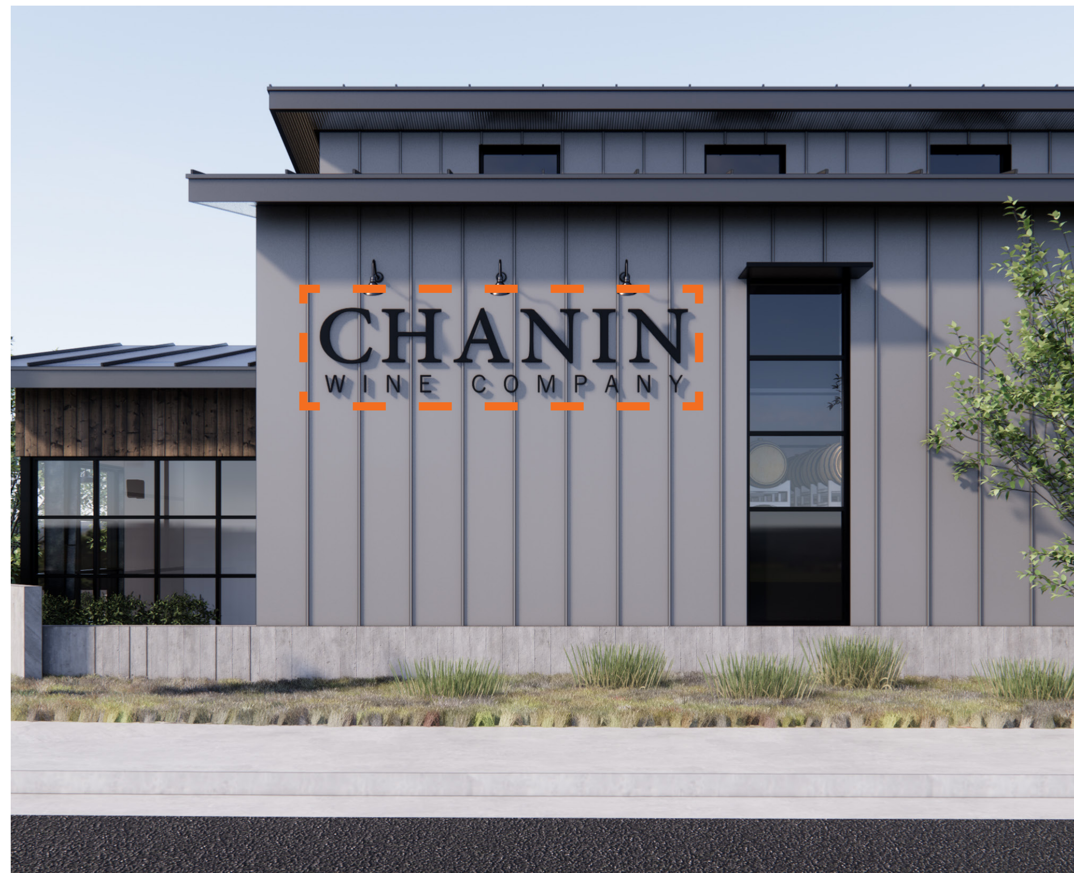
WALL SIGN #1 Insulated metal panel building wall 14'-6" wide x 3'-6" tall cut steel logo lettering with LED 'sign' lighting, fixture B2 51 sf sign area
