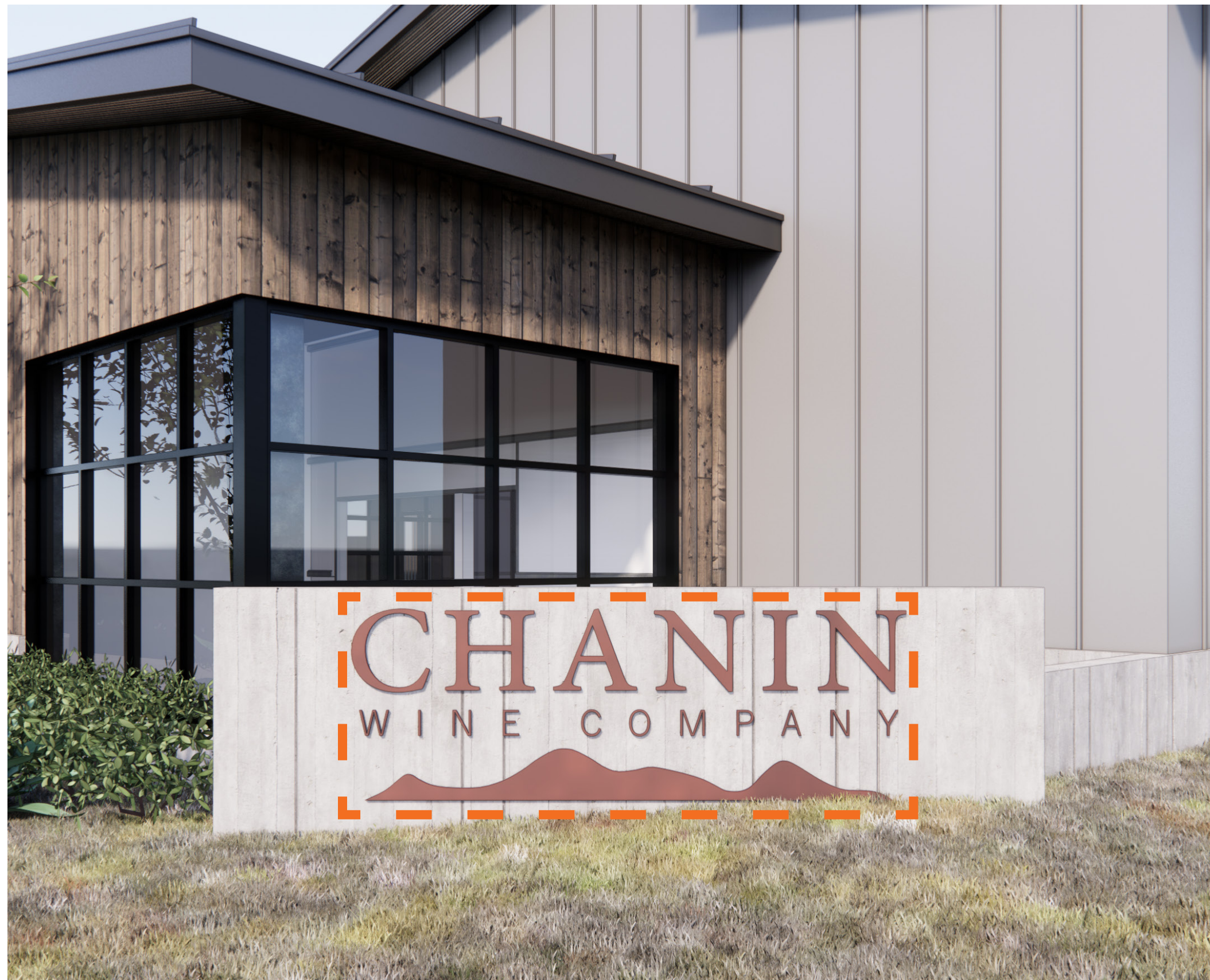
MONUMENT SIGN #1 13'-4" wide x 4'-4" tall cast-in-place concrete monument, meets minimum 5' setback 9'-0" wide x 3'-0" tall cut steel logo lettering with LED 'halo' backlighting 27 sf sign area
