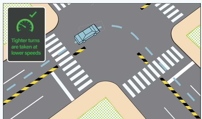
With left turn traffic calm in place along the roadway centerline, a vehicle makes a proper left turn following a safe path.
