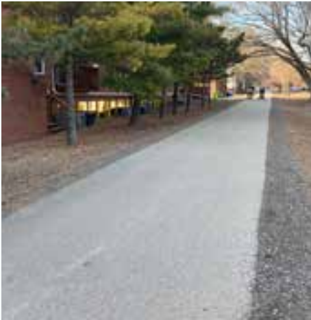
Segment of Constitution Trail with asphalt and crushed gravel shoulders in Normal, Illinois
