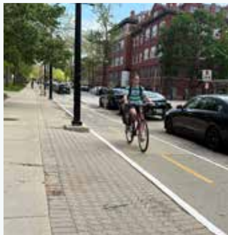
A bicyclist on a striped bi-directional bike lane which is between parked cars and brick pavers along a sidewalk at University of Illinois in Urbana-Champaign, Illinois
