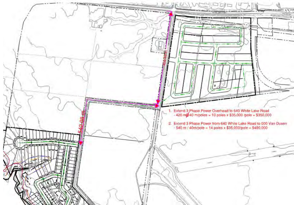
Figure 14 Hydro One Extension of Servies
