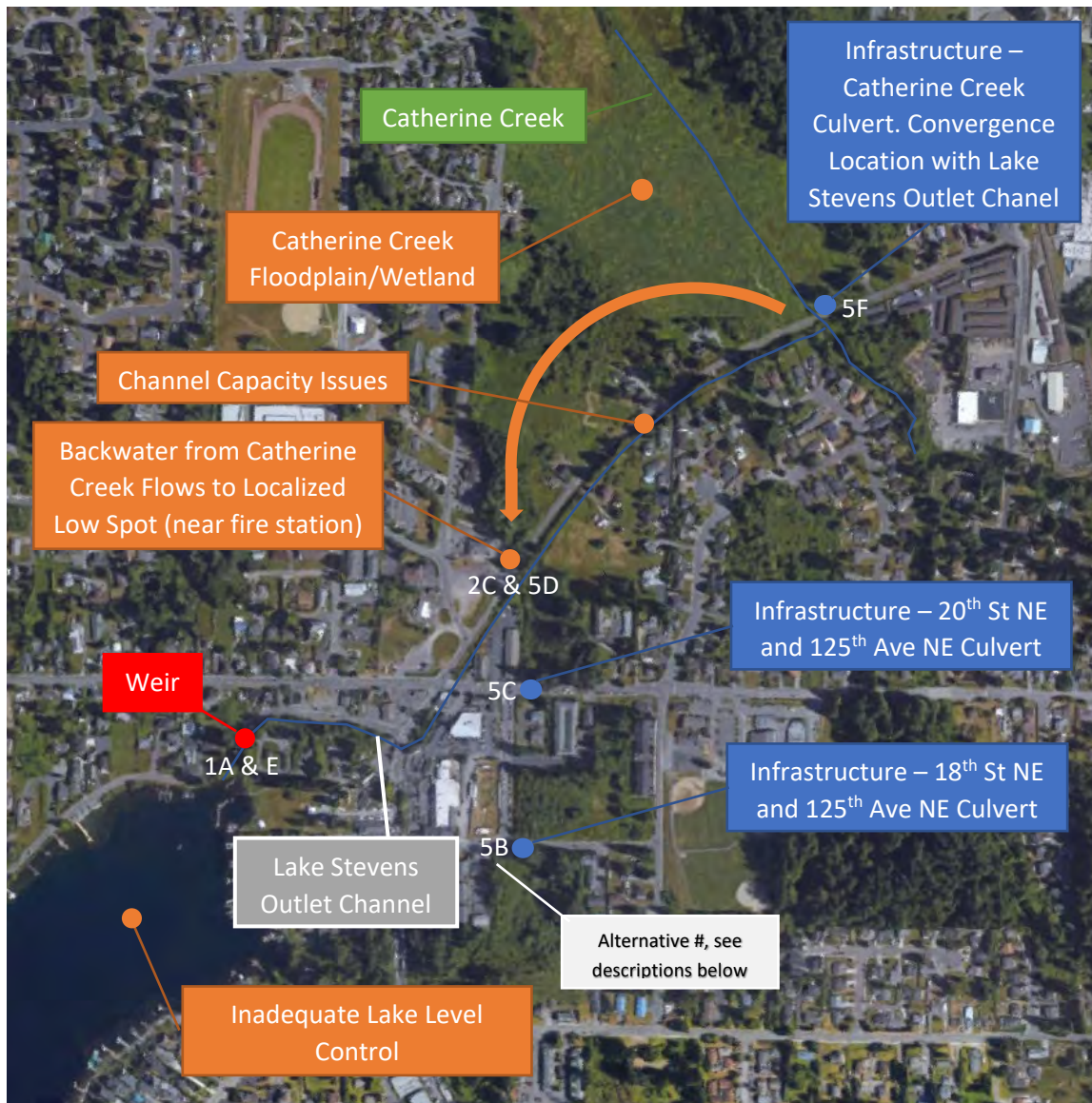
Figure ES-1. Lake Stevens Outlet Channel existing conditions
