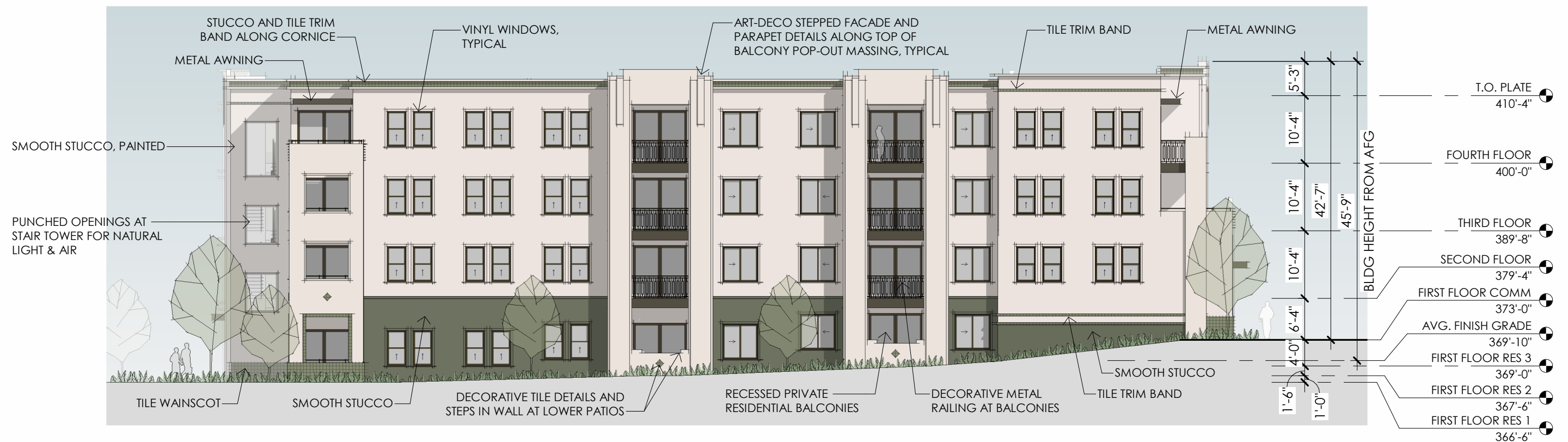
SIDE ELEVATION (NORTH)
