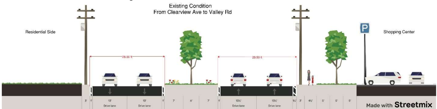
Figure 6: Typical Section - Existing Condition (Looking Northbound)
